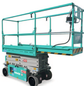
Extensie platforma 1 m
